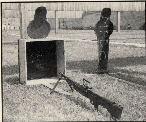
M60 in 7.62 loaded with Simunition's Lead Free Frangible Ammunition was fired nearly point blank at steel plate to demonstrate there is no splashback or ricochet.
